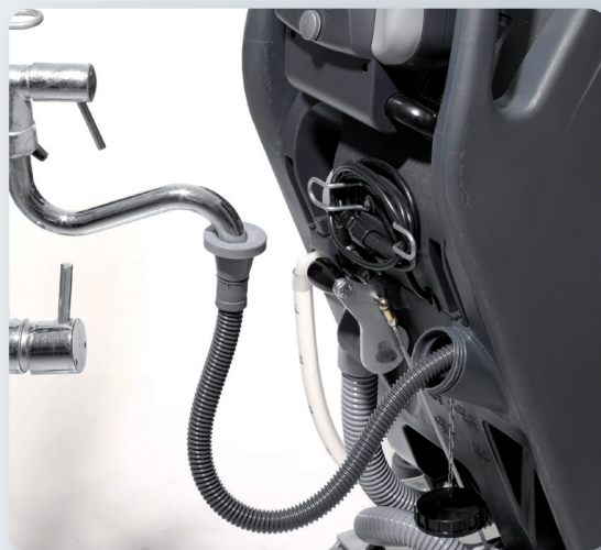
Easy-fill tank system utilizes an integrated hose. Allowing the machine to be filled from the nearest available water tap, and reduces downtime considerably (optional)
